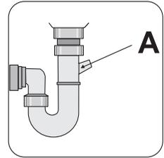
When connecting the drain hose to an under sink trap spigot, **the entire plastic membrane (A) must be removed**. Failure to remove all the membrane will result in food particles building up over time eventually blocking the dishwasher drain hose spigot.
