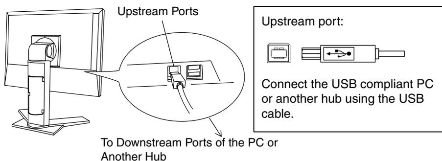
After connecting the USB cable, the USB function can be set up automatically.
