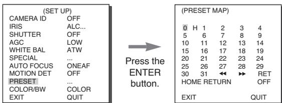
You can store up to 128 ZOOM and FOCUS positions with the PRESET. You can use the PRESET function when you connect the SSC-1000 to the RS-485.
