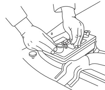
11. Ground amplifier to chassis of vehicle; connect the terminal provided to the 10ga black wire from furnished wiring harness. A good ground is as important as the power connection. The ground should be as short as possible and the contact point should be free of paint and debris.
