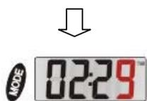
After finishing the timer setup, press the "MODE" button to start the countdown.
