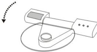
**STEP 2:** Press the “ON/TARE” button and the scale will display “HELO”, and then zero. The scale is now ready for weighing.
