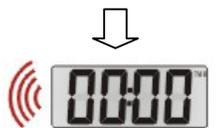
After finishing the countdown, "00.00" will appear on the LCD display and alarm will sound.
