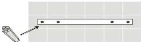
**STEP 3:** Install the fixture plates to the holes and drill in the screws tightly to secure the
