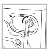
of the water inlet hose to the washing machine, screwing it onto the appliance's cold water inlet, situated on the top right-hand side on the rear of the appliance (see figure).
