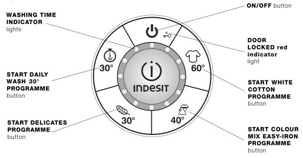
**ON/OFF** button: press this to switch the machine on or off. When the machine is switched on, the buttons used to start various programmes begin to flash, while the washing time indicator lights illuminate in a fixed manner.
