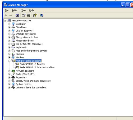
5. In the Device Manager window, click on the Multiport serial adapters icon to display the currently installed devices.
