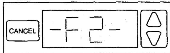
A fault code indicates that there may be a functional error. As a safety precaution, the control will automatically cancel the program. Follow the procedures described below to check the wall oven.
