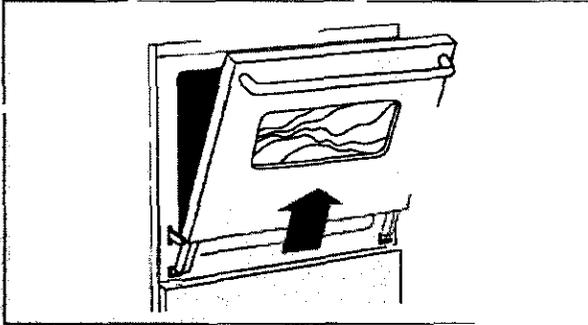
**CAUTION:** Hinge arms are spring mounted and will slam shut against the oven if accidentally hit. **Never place your hand or fingers between the hinges and the front oven frame.** You could be injured if the hinge snaps back.
