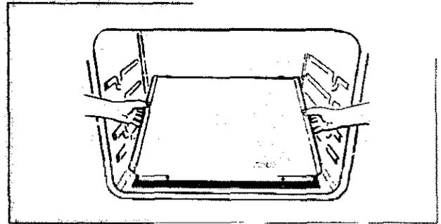
**To replace:** Fit the rear edge of oven bottom into the pin located at the center of the channel on the rear oven wall. Push toward the rear of the oven and lower oven bottom into place.
