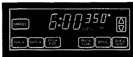
The oven will turn on at 3:30, cook the food for 2-1/2 hours and will automatically turn off at 6:00. Press the CANCEL pad to stop the beeps.
