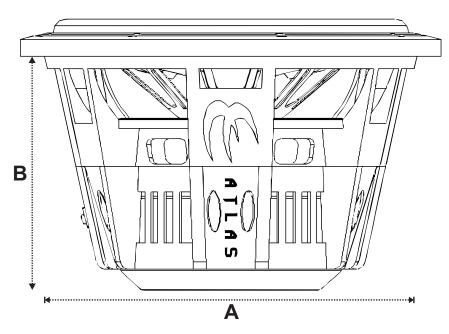
Due to the vented backplate, you must allow for an additional 2" behind the subwoofer when designing your speaker enclosure.
