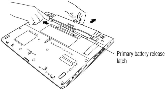
*(Sample Illustration) Unlocking the battery release latch*
