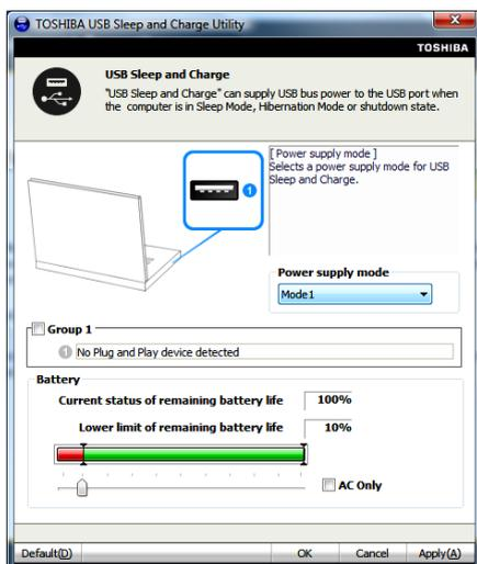
In this situation, select a different mode. “USB Sleep and Charge function” may not be functional with some connected external devices even if the appropriate group is selected. In this situation, uncheck the check box for the group and discontinue using this function.
