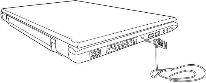
*(Sample Illustration) Attaching security lock cable*
