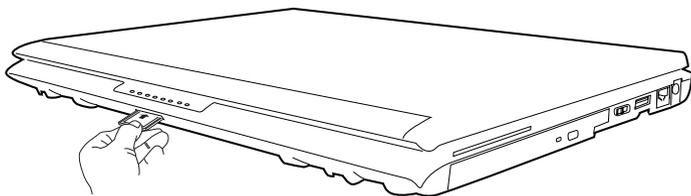
*(Sample Illustration) Inserting an SD card*
