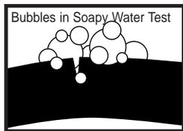
DURING ANY PORTION OF THE SOAPY WATER TEST, IF BUBBLES CONTINUE TO APPEAR, STOP, DO NOT USE THE GRILL AND CONTACT YOUR LOCAL PROPANE DEALER OR MASTERBUILT AT 800-489-1581 NOTE: USE A 20 LB. CYLINDER OR SMALLER WITH A PROTECTIVE COLLAR WITH THIS GRILL.
