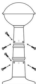
1) Mount center post first to the base and secure with three screws.
