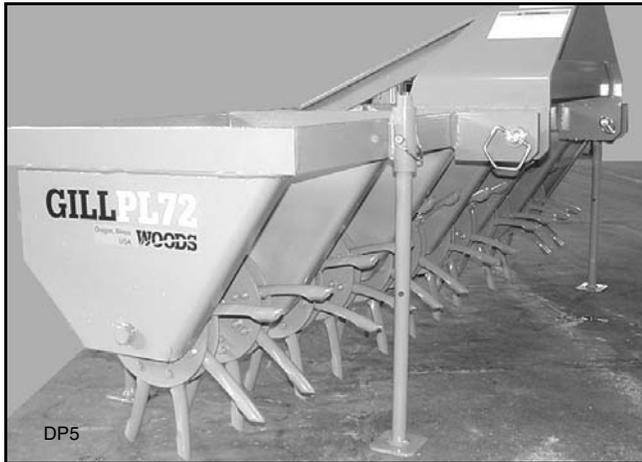
**Figure 6.** Parking Stands Lowered into Storage Position
