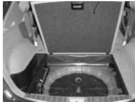
**STEP 2:** Open the cargo flooring and hook it to the upper lip of the tailgate opening. Remove the organizer tray, wooden board, factory woofer enclosure, spare tire and the driver's side cargo pocket cover.
