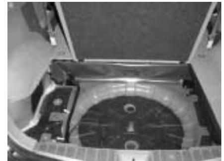
**STEP 3:** a) With a Phillips® screw driver, remove the driver's side cargo pocket.
