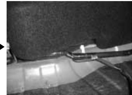
**STEP 7:** There is a large L-bracket that is already mounted to the rear of the Stealthbox®. This L-bracket needs to be unmounted, flipped around and remounted. The picture above shows the large L-bracket properly mounted, with the woofer facing down.
