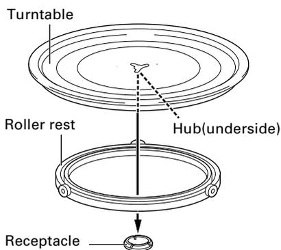
1. Place the roller rest on the cavity bottom.
