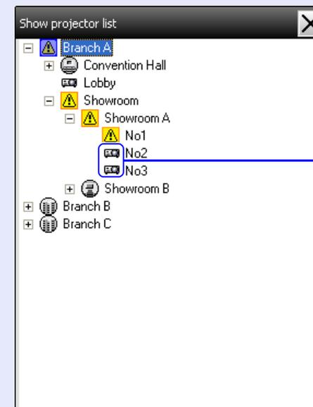
With "Projector list", temperature level icons are not displayed regardless of the setting of "Temperature level display group view" at "Environment setup".
