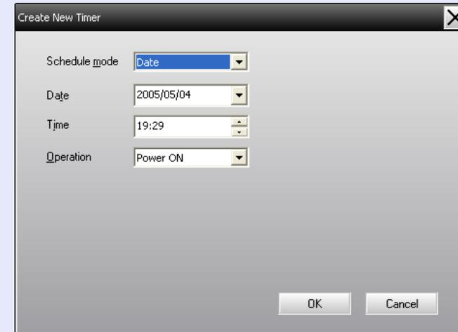
At "Operation", you can carry out the operations of turning the power on and off and switching the input sources, similarly for the control buttons on the main window. If you set the input source switching, the projector's power will turn on at the timer start time even if it is not on at the time. Because of this, it is not necessary to make two separate timer settings for turning the power on and switching the input source.
