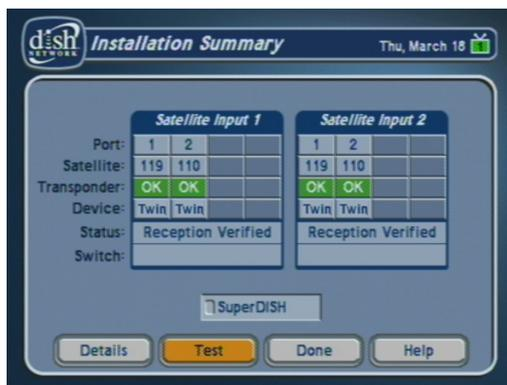
6. Make sure that the information on the **Installation Summary** screen identifies your system correctly and shows all transponders for all satellites in your system. Your screen may look different from the example above depending on the dish antenna system you are using.
