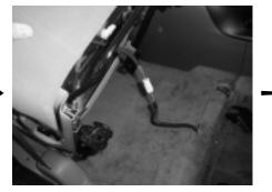
**STEP 2:** Tilt the seat to the rear, unplug the exposed wire assembly, remove the seat from the truck.
