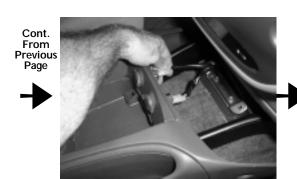
**STEP 7:** Slide the center console to the rear of truck. This will allow exposer of the 12v plug wires. Unplug and then remove the center console from truck
