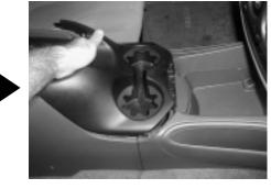
**STEP 4:** With the main storage door open, grab ahold of the black cup holder section and pull up.
