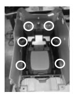
**STEP 9:** Remove the 8 screws that is securing the black plastic support to the outer console. Not all circles represent all 8 screws.
