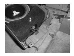
**STEP 21:** Place the Stealthbox/center console into vehicle. Attach the speaker wire to terminal.
