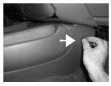
**STEP 6:** Remove the plastic buttons that are located on each side of the center console.
