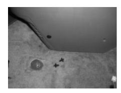
**STEP 22:** Place Stealthbox/center console upright and into the proper position. Carefully guiding the threaded rods through the three drilled holes.
