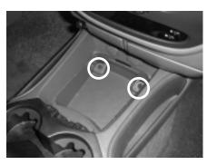
**STEP 3:** Remove the front storage access door. Using a 10mm socket, remove the exposed bolts.
