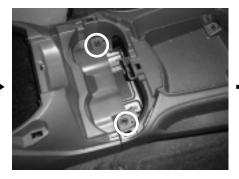
**STEP 5:** Using a 10mm socket, remove the exposed bolts. Also remove the bolts that are located at the bottom of the main storage bucket.
