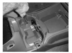
STEP 24: With the Stealthbox securely mounted to the vehicle. Secure the plastic console to the floor, using the factory screws from **STEP 5**.
