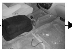
**STEP 19:** With the Stealthbox and the modified A/C ducts in position. Place the front section of the center console back into the proper location. Do not secure at this time.
