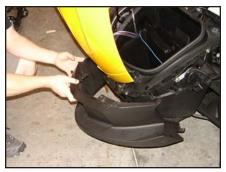
**STEP 5**Remove the front Air dam.
