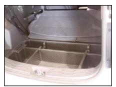
Lift the floor, remove the compartmented foam spacer this will not remain in the vehicle.
