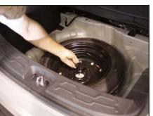
Remove the tool kit that resides inside the spare tire and the spare tire itself, set aside the hardware as it will be re-used.
