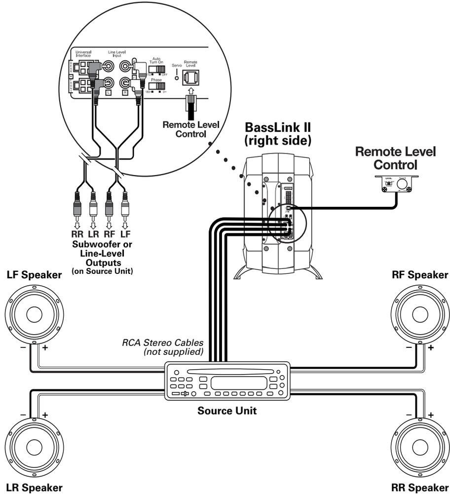
Figure 8. BassLink II audio connections for a head unit equipped with four speaker-level outputs.
