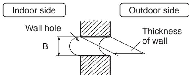
(Section of wall hole) © Piping hole pipe
