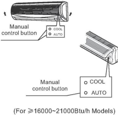
1. Open and lift the front panel up until it remains fixed with a clicking sound.
