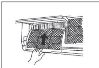
4. Remove the air-freshening filter from its support frame (The installation and removal method of the air-freshening filter is different depending on the models (see pictures marked as 1 and 2 on the left).
