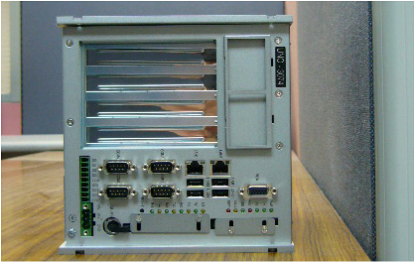
Figure 3.6: UNO-3074 Improper Installation (1)
