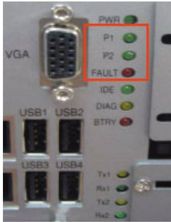
Figure 2.12: LED Locations to Monitor Power Input
