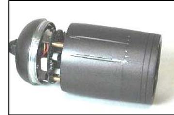
1. Turn camera housing counter clockwise to remove
