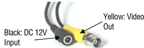
The 6 ft camera cable has a female BNC connector (for video output) and a female power jack
