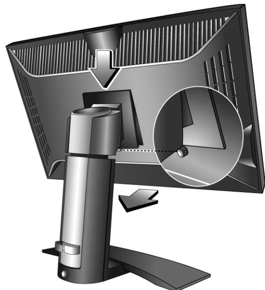
3. Fully extend and tilt the monitor to rotate it.
