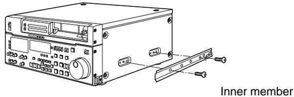
The length of the screws used is subject to restriction. Use screws which are less than 2/5" long in their place.
