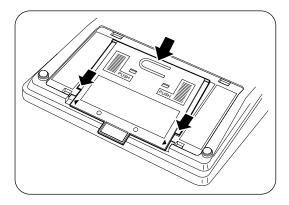
**2** While pushing on the areas marked "PUSH", insert the edges of the holder under the slide rails and then slide in the direction of arrow (A).
