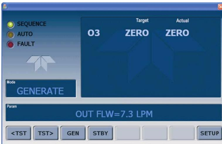
**Figure 3-2: Display Screen and Touch Control**
