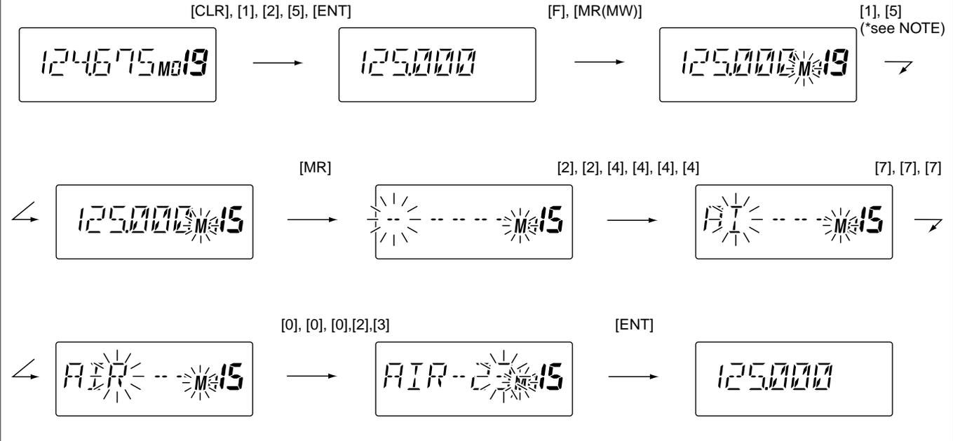
**\*NOTE:** Push [BANK], then rotate the [DIAL] to select the BANK number, if desired. Push [CLR] to continue memory name programming.
