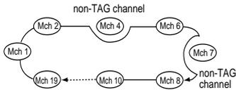
Repeatedly scans all “TAG” memory channels. Used for checking often-used channels and bypassing usually busy channels such as control-tower frequencies..
