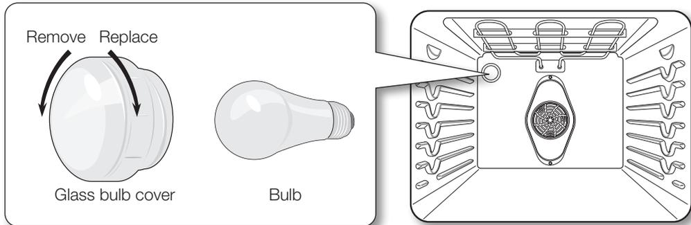
5. Replace the light bulb and glass bulb cover by turning them clockwise.
