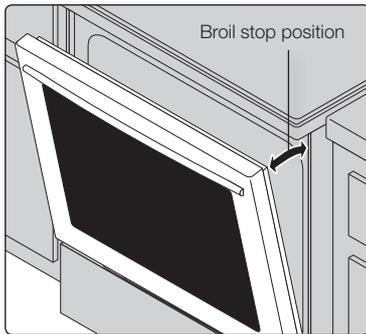
Leave the door open at the broil stop position. The door will stay open by itself, yet the proper temperature is maintained in the oven.
