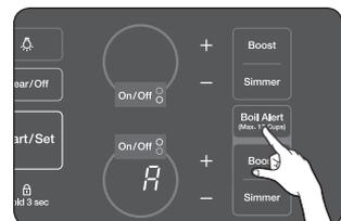
3. Touch the +/- pads to select the power level you want the element set to after the water boils.
