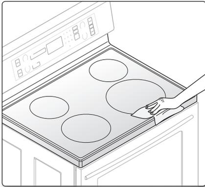
To clean the seal around the edges of the glass, lay a wet cloth on it for a few minutes, then wipe clean with a nonabrasive cleaner.
