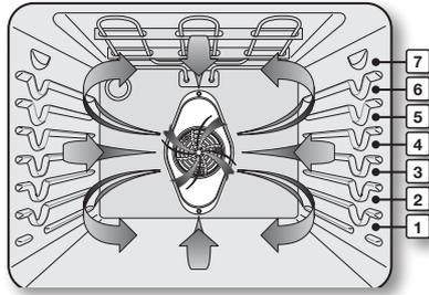
By using the convection bake feature, you will be able to cook faster. You can program the oven for convection baking at any temperature between 150°F and 550°F.
