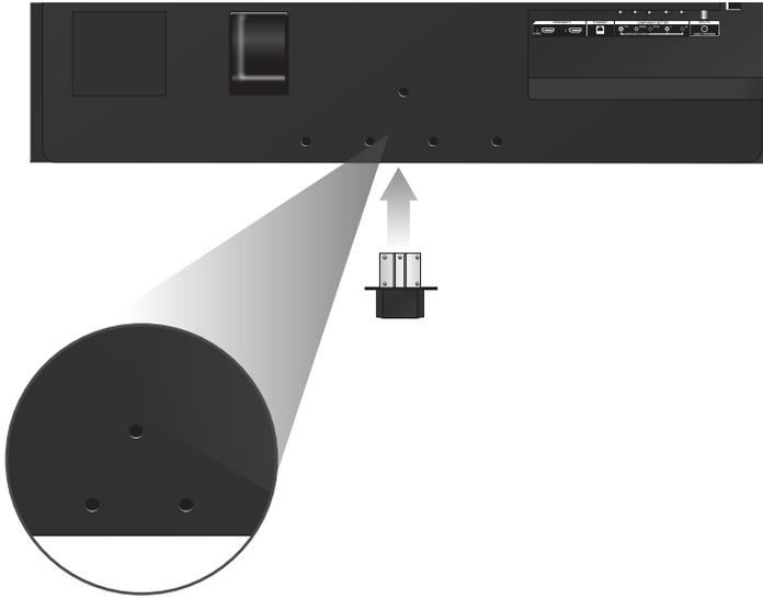
Align the neck piece with the bottom of the TV and slide it into place as shown.
