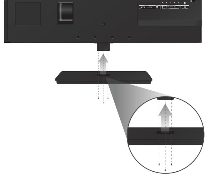
Align the base with the neck and tighten three (3) M4 14mm screws using a philips screwdriver.
