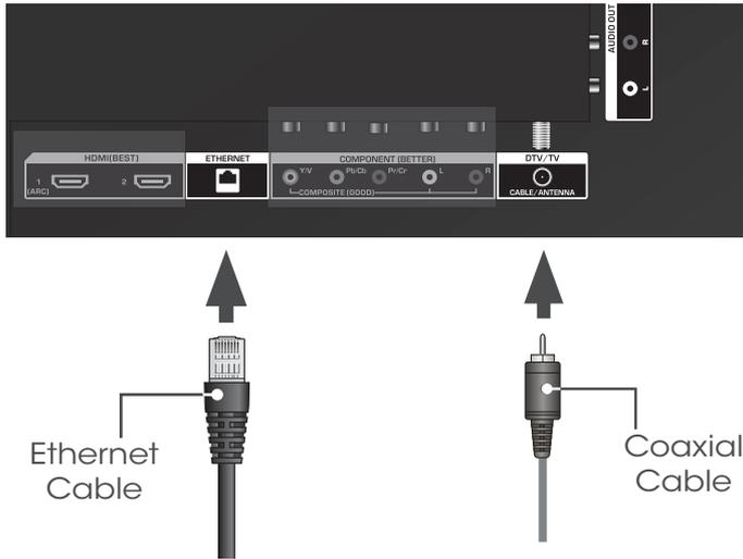
If you have an external antenna or a cable connection that extends from a wall outlet, connect it to the TV with an RF/Coaxial cable.
