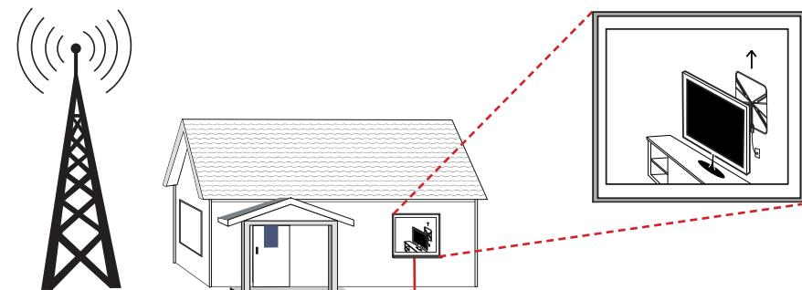
Electronics may reflect the signal from the broadcast tower. If so, try mounting the antenna higher on the wall, and run a new channel scan. The higher the antenna, the better signal you will receive.
