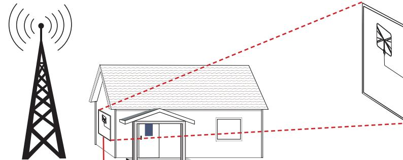
If the antenna is mounted so that it hangs vertically, the coax cable should run from the top or bottom of the antenna.
