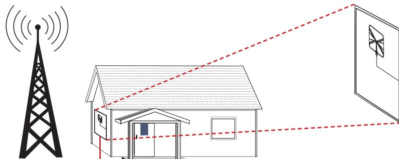
Mount the antenna on a window that faces the broadcast tower of stations that you want to receive. The sides of the antenna may not "see" enough signal from the broadcast tower if the sides of the antenna face the tower.
