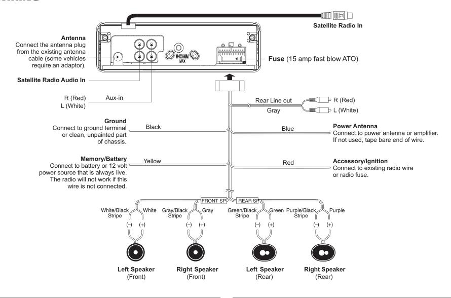
NOTE: The amplifier in this radio is only designed for use with four speakers. Never combine (bridge) outputs for use with two speakers. Never ground negative speaker leads to chassis ground. Failure to wire exactly as shown may cause electrical damage to the radio.
