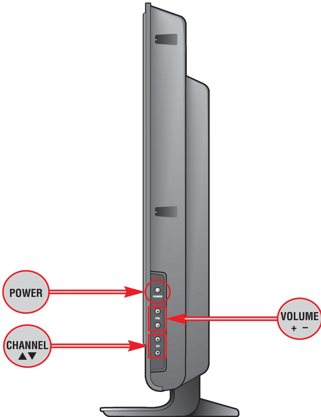
These keys operate exactly like the Remote Control keys.
