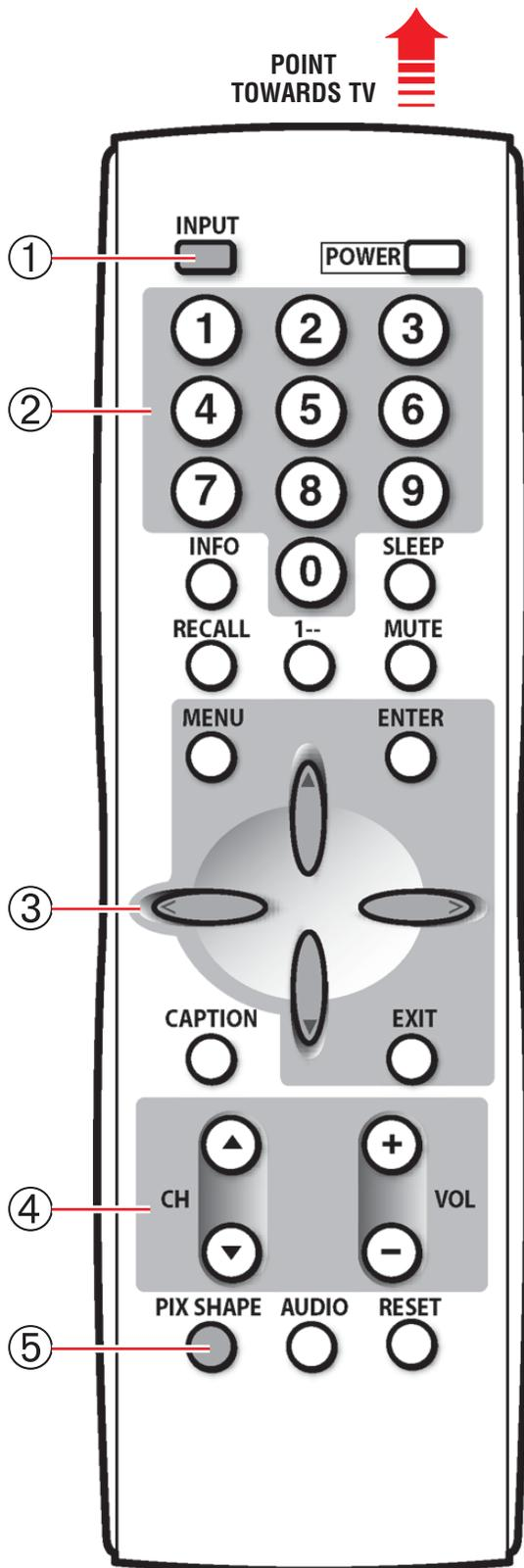
① **Input Key**—Press to select the program source to watch: Analog RF ➔ Digital RF ➔ Video 1 ➔ Video 2 ➔ Video 3 ➔ HDMI 1 ➔ HDMI 2 ➔ HDMI 3 ➔ Analog RF.
