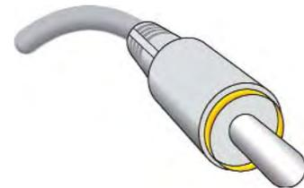
**Composite Audio/Video (RCA type)**—Use these cables for standard analog audio/video connections. Normally cables are color coded: Yellow for Video, White for (L) Audio, and Red for (R) Audio.
