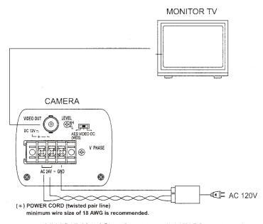
24V AC UL Listed Class 2 power supply / 12V DC power supply
