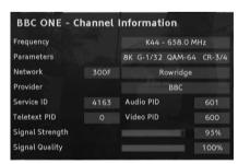
4 Adjust your antenna so that the two specifications **signal strength** and **signal quality** display a preferably high value.
