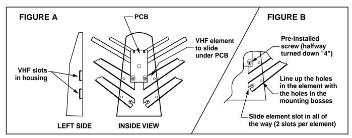
STEP 3: After the elements are totally in place, tighten the two pre-installed screws. Tighten to the point where the element and PCB feel tight. Do not over tighten. This may result in stripping threads.
