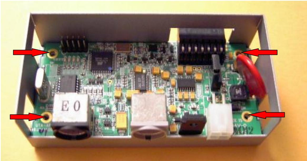
Remove the top, and remove the pc board inside
