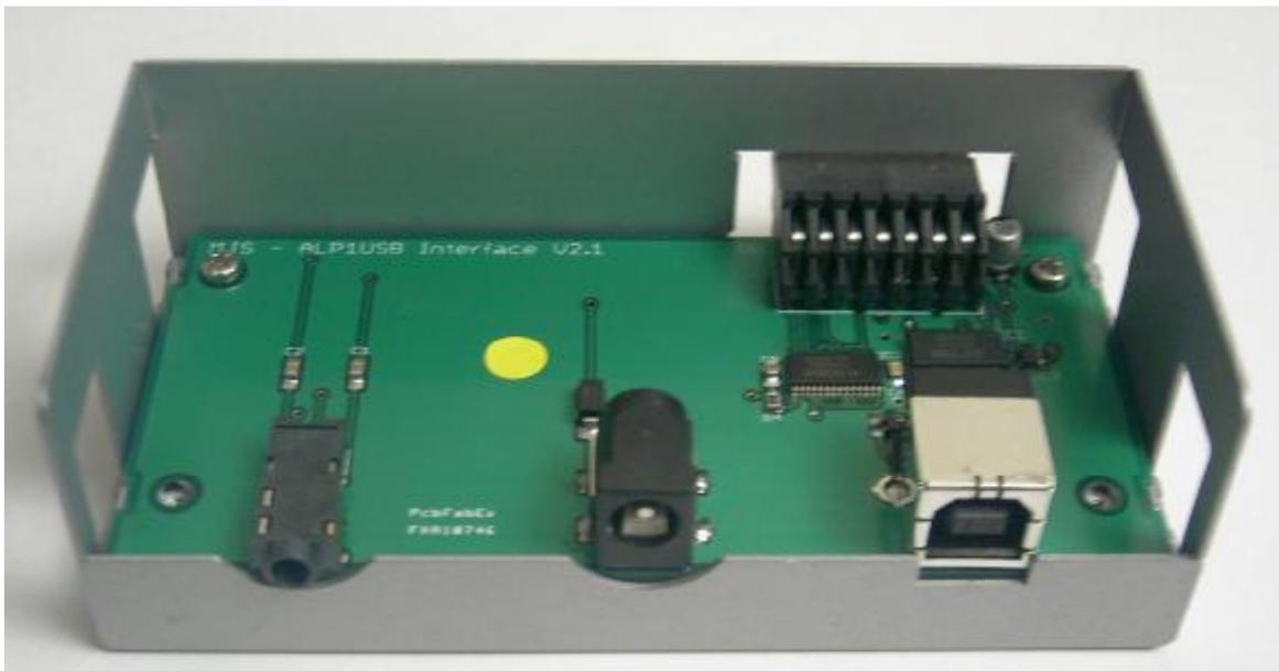
Install the new board. Secure with same screws.
