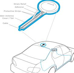
Not properly placing or installing the antenna can create safety hazards during an accident.
