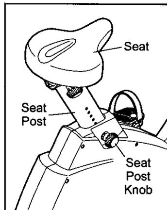
to loosen it (if the knob is not loosened enough, it may scratch the seat post). Next, pull the knob, slide the seat post to the desired height, and then release the knob. **Move the seat post up and down slightly until the pin on the knob snaps into one of the holes in the seat post.** Then, turn the knob clockwise until it is tight.
