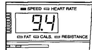
Note: The console can display speed and distance in either miles or kilometers. To find which unit of measurement is selected, you must select the console's user mode. Hold down the Program Select button for about three seconds. The letter "E" for English miles or the letter "M" for metric kilometers will appear in the left display. To change the unit of measurement, press the + button.
