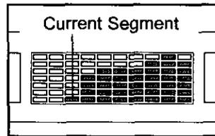
When only three seconds remain in the first segment, both the Current Segment column and the column to the right will flash, a series of tones will sound, and *all resistance settings will move one column to the left*. The resistance setting for the second segment will then be shown in the flashing Current Segment column and the resistance of the exercise cycle will automatically adjust to the resistance setting for the second segment.
