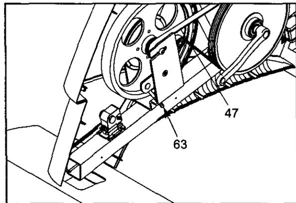
Next, turn the indicated M8 Nylon Locknut (63) until the Drive Belt (47) is properly tightened. Then, reattach the side shields.
