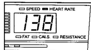
appear in the right display, and then your heart rate will be shown. For the most accurate heart rate reading, continue to hold the contacts for about 15 seconds. Note: If your heart rate is not shown, make sure that your hands are positioned as described. Be careful not to move your hands excessively or to squeeze the metal contacts too tightly.
