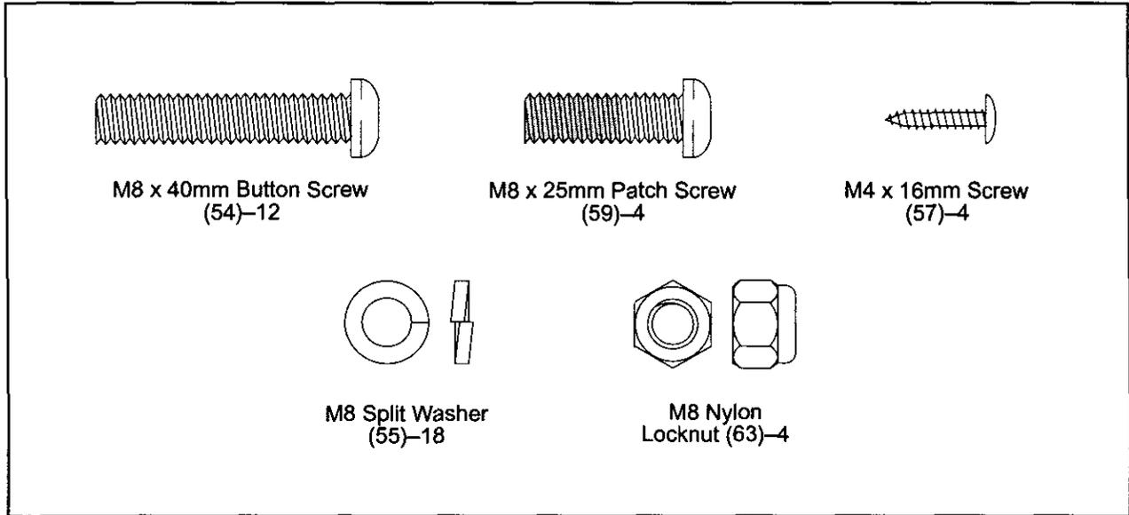
1. Identify the Front Stabilizer (15). While another person lifts the front of the Frame (1), attach the Front Stabilizer to the Frame with four M8 x 40mm Button Screws (54) and four M8 Split Washers (55).
