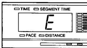
While the user mode is selected, press the Program Start button. The left display will then show the total number of hours that the exercise cycle has been used. Press the Program Start button again. The left display will then show the total number of miles pedaled. To exit the user mode, press the Program Select button again.
