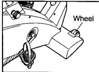
If the exercise cycle rocks slightly during use, turn the leveling feet under the rear stabilizer until the rocking motion is eliminated.
