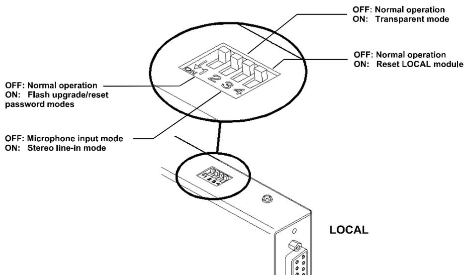
*Note: When shipped, all switches are set in the OFF positions and this will produce normal operation with normal microphone input (at the REMOTE module.)*
