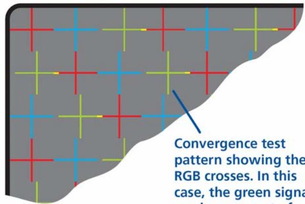
**Convergence test pattern showing the RGB crosses. In this case, the green signal can be seen out of line with the other two colours.**
