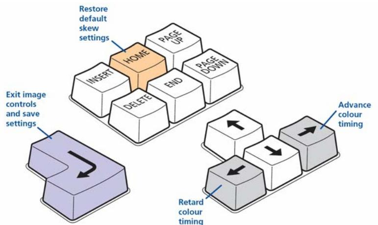
*Note: Once you have made a skew adjustment, it may be necessary to re-adjust the image controls to attain an optimum screen image.*
