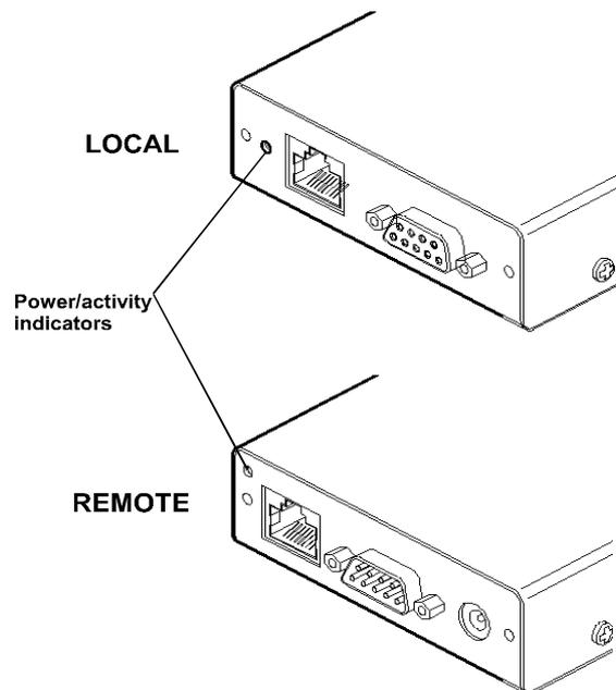
*Note: Both modules contain internal automatic cut-out fuses to protect against power surges. To reset, remove power (or, for the LOCAL module, the keyboard connection) from the module for one second and then reconnect.*
