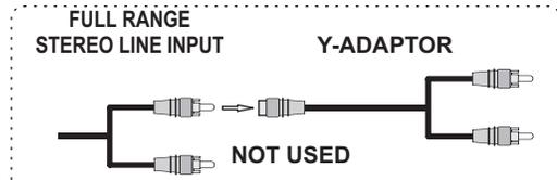
Note: You can use the Radio/CD designated mono line output or a full range stereo line output. For full range stereo line output, you will need an optional "Y-Adaptor" as shown.
