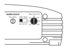
I) "Filter Mode" Control: The e1200 employs a 12dB per octave filter. This filter can be configured into one of two filter types or defeated completely by way of the three-position "Filter Mode" switch: "Off": Defeats the filter completely, allowing the full range of frequencies present at the inputs to feed the amplifier. This is useful for systems utilizing outboard crossovers or requiring full-range reproduction from the e1200.
