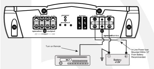
**IMPORTANT!** Before making any connections, disconnect the car's battery until the installation is completed to avoid possible damage to the electrical system.
