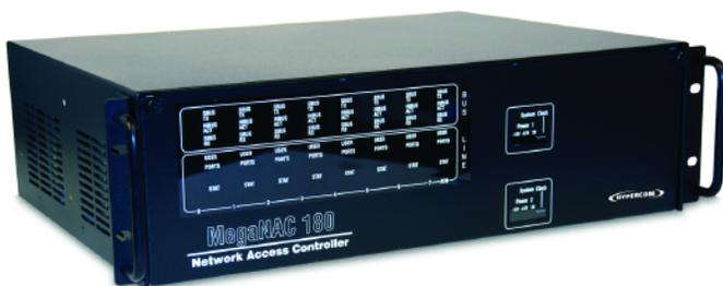
**Multi-protocol** ► POS dial access termination for up to six T1/E1s
