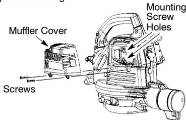
1. Loosen and remove the 2 screws from the muffler cover.
