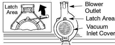
3. Gently tilt the handle of the screwdriver toward the back of the unit to release the latch while pulling up on the vacuum inlet cover with your other hand.
