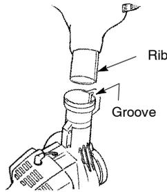
5. Insert the elbow tube into the blower outlet. Make sure elbow tube rib is aligned with the blower outlet groove.
