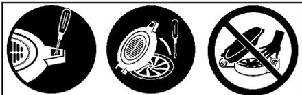
**⚠ WARNING:** Stop the engine before opening the vacuum inlet door. The engine must be stopped and the impeller blades no longer turning to avoid serious injury from the rotating blades. Gently tilt the handle of the screwdriver toward the back of the unit to release the latch while pulling up on the vacuum inlet cover with your other hand.
