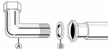
**Warning:** if you use a stainless steel flexible pipe, it must be installed in such a way that it does not come into contact with moving cabinetry like drawers or kitchen cupboards and passes at a point free of obstacles where it can be examined in its entirety.
