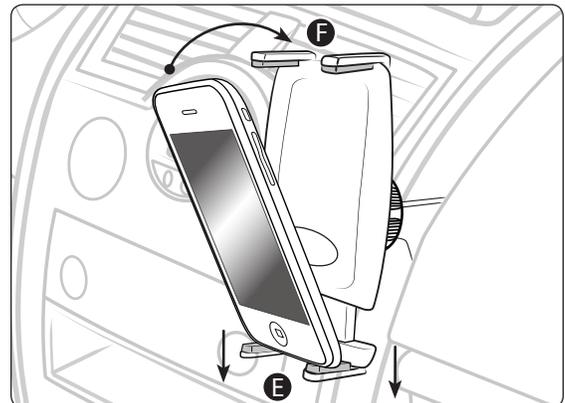
\* If necessary, install the (2) extra long support legs (SP-SM050-LF) to accommodate large sized phones.
