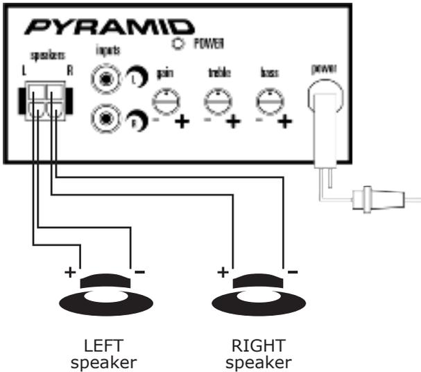
**NOTE: The PB440X is not capable of having bridged outputs. Bridging the outputs will damage your amplifier!**
