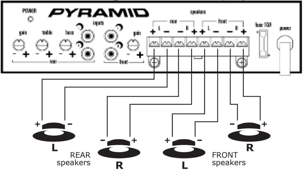
**NOTE: The PB442X is not capable of having bridged outputs. Bridging the outputs will damage your amplifier!**
