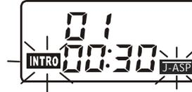
3.) Press the STOP ■ button to stop the disc and then press the PLAY/PAUSE ►|| button again. The "INTRO" indicator stops flashing and remains 'On'. The player returns to the beginning of track 1 and plays just the first 10 seconds of each track on the disc. When the first 10 seconds of each track has been played, the player stops.
